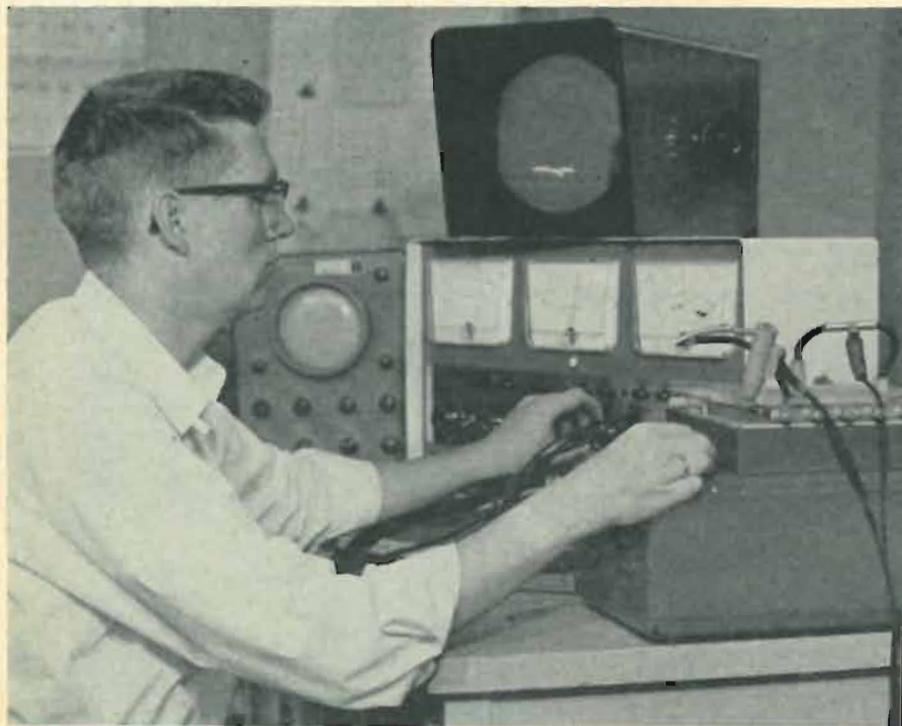
Automotive electronics specialist Paul Strycker completes final checkout of scope-type ignition analyzer. Unit is used, but seldom repaired, by auto mechanics.
