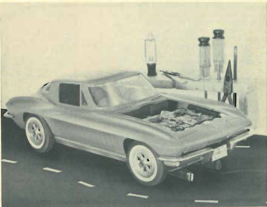
Scale-model car has two transistor receivers in the engine compartment. Loopstick antennas protrude beneath front bumper, pick up signal from road antenna.
