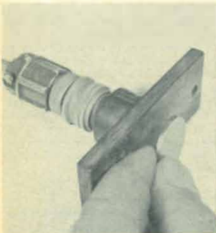
Presence of metal coin increases eddy-current losses of coil, stopping oscillator.
