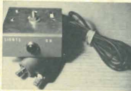
One holding screw on unit is needed to secure assembly to the dashboard. For a fast connection to the wires under dash, use insulation-piercing alligator clips.
