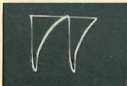
Fig. 4—Direct probe distorts signal (a). Lo-cap probe produces normal pattern (b).
